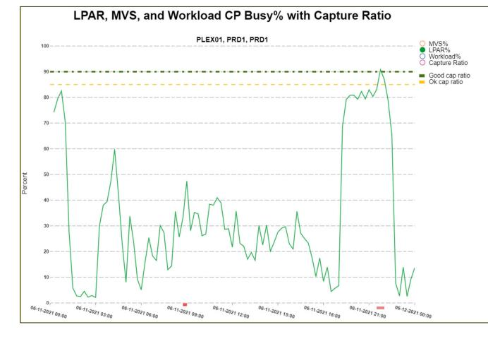
When the number of logical processors assigned to a partition is equal to the number of physical processors on the CEC, the LPAR utilization for that LPAR will equal the physical utilization for that LPAR.
