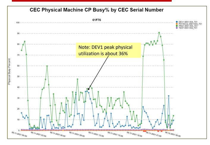
For each logical partition, the physical utilization of the machine is a function of the number of physical processors.
