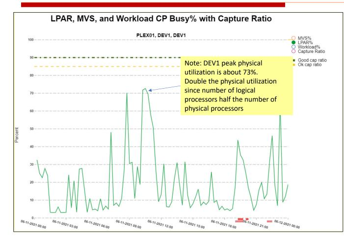
When the number of logical processors assigned to a partition is NOT equal to the number of physical processors on the CEC, the LPAR utilization for that LPAR will be higher since we are looking at the constraint of the number of logical processors.
