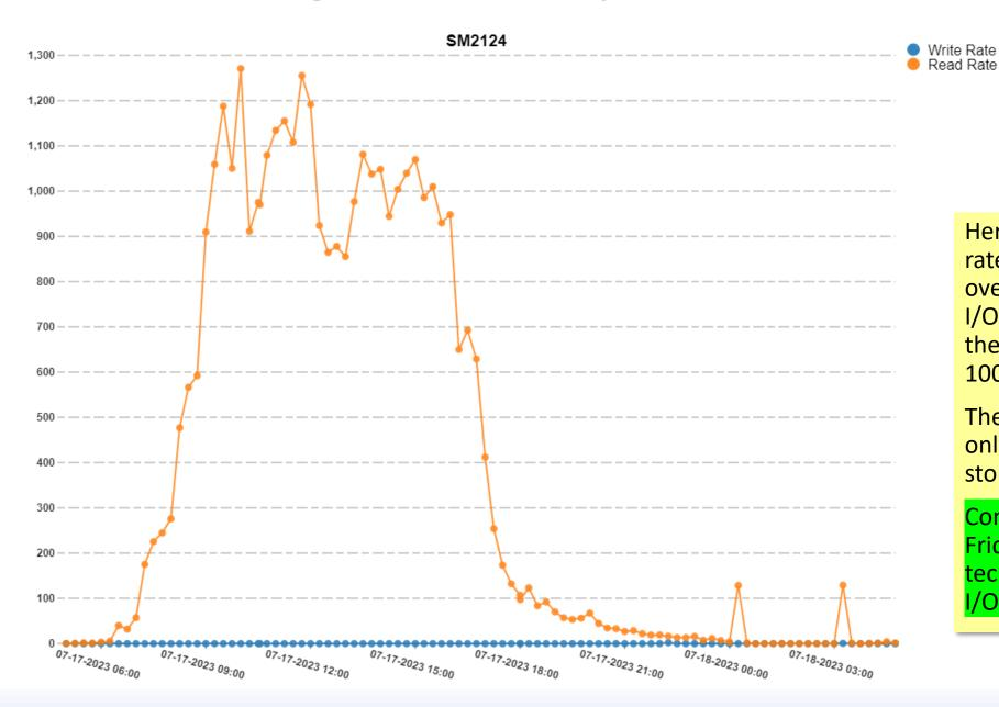
Here's the read and write rate for a particular volume over time. Virtually all the I/O is read I/O, and during the day it is doing over 1000 IOPS.
