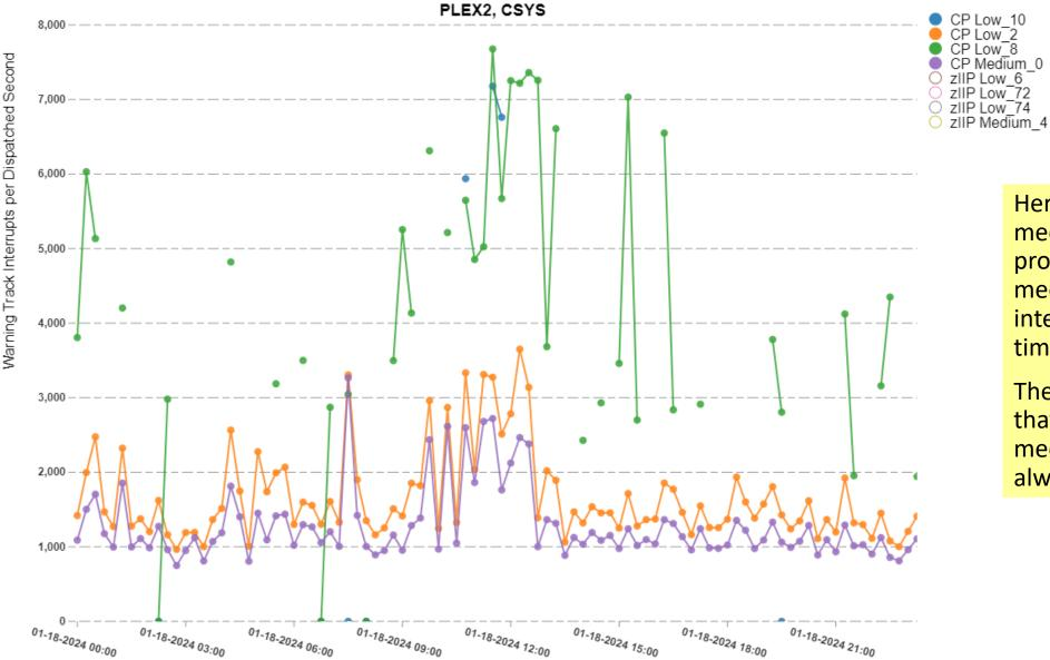
Here this LPAR only has medium and low pool processors, and the medium is getting interrupted over 1000 times / second.
