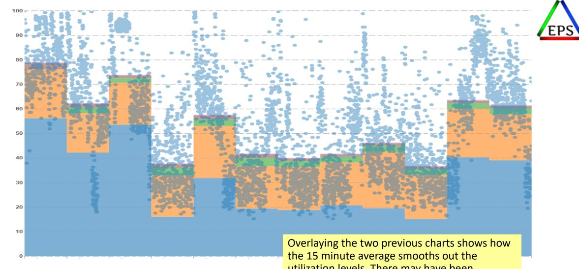
Overlaying the two previous charts shows how the 15 minute average smooths out the utilization levels. There may have been performance issues due to running at or nearly 100% busy at times, but that's really lost in the 15 minute averages.
