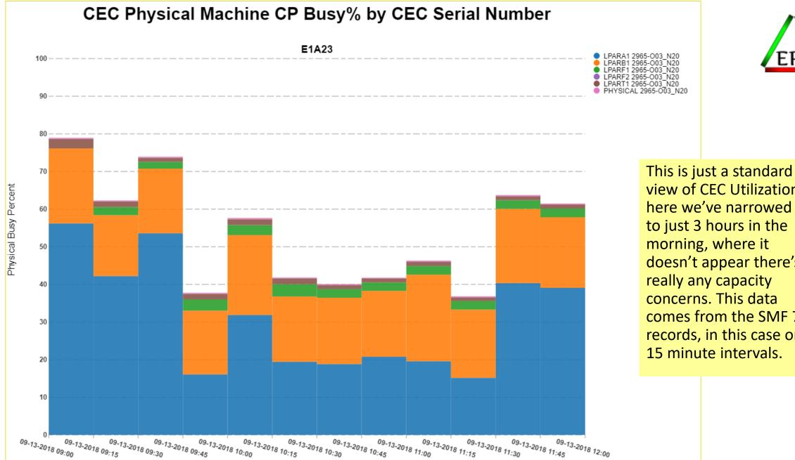
view of CEC Utilization, here we've narrowed in to just 3 hours in the morning, where it doesn't appear there's really any capacity concerns. This data comes from the SMF 70 records, in this case on 15 minute intervals.
