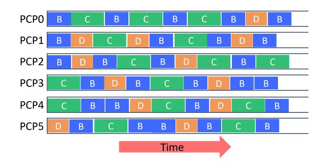
PR/SM time slices the physical processors dispatching logical to physicals for specific durations (or until the LPAR gives back the processor). With Horizontal CPU management, a logical CP might get redispatched to any physical CP.
