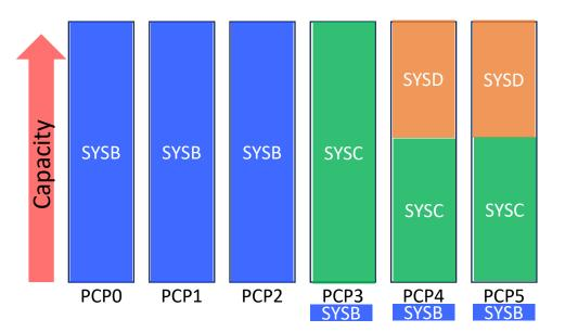
With vertical CPU management, this is closer to reality. Note that SYSB's VLs will only come into play when there's both demand from SYSB and the others' aren't using the capacity.
