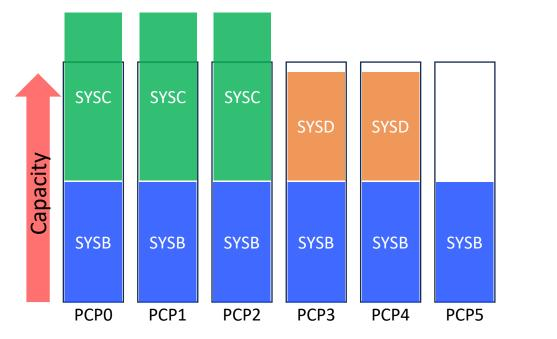
Note that capacity for the LPAR is spread horizontally across all the LCPs. Although in reality, PR/SM wouldn't (couldn't!) statically allocate logicals to physicals like this.
